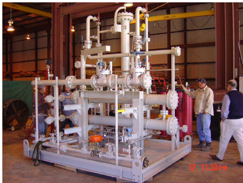
Figure 8. Membrane-based FGCU installed on Kakap-H remote natural gas platform, Indonesia.
