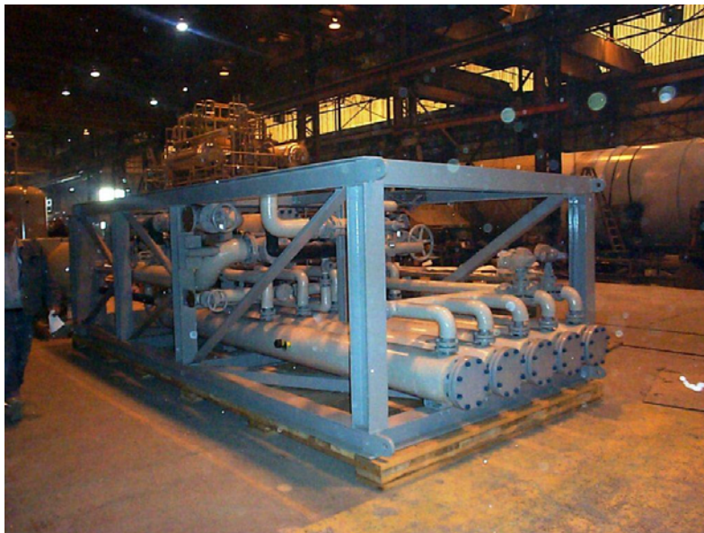
Figure 10. Membrane-based FGCU prior to installation on a North Sea FPSO ship. The unit was installed with the module tubes in a vertical position (perpendicular to the ship deck), in order to minimize the footprint of the unit.
